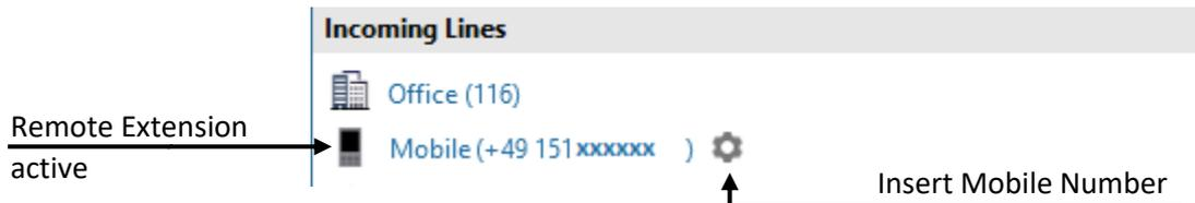
If the **Remote Extension** is active, incoming calls can be accepted on the deposited mobile phone.
